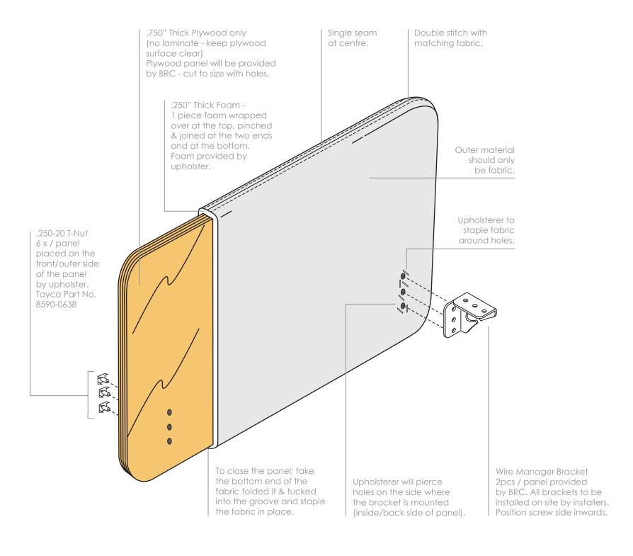
Finish Thickness 1.250" Tol. +/- .075" Line the end of the top flat part of the bracket to create a .500" gap between the panel & work surface. Work Surface .250"-20 x .625" Panhead socket screw 6x for each panel assem. Panhead socket # 10, .750"Len. wood screw 6x for each panel assem.
