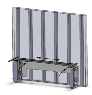
5 Place the entire assembly up against the wall and locate as desired.
