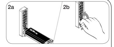
To unlock: Insert a valid Manager Key then turn the knob to the unlocked position. Open the door.\*\*
