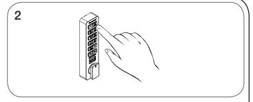
While the LED is on, enter the number of hours from 1 - 99 then press  $\overline{\mbox{\mbox{$\mbox{$\cdots$}}}}$ .
