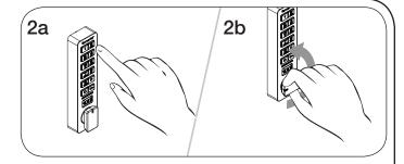
To unlock: Press © [the same 4-7 digit code] @ then turn the knob to the unlocked position. Open the door.\*
