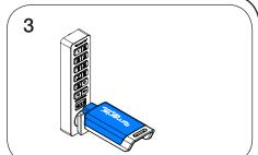
While the LED is on, insert a new User Key. Two sets of two-tone beeps will be heard and the LED will turn off.
