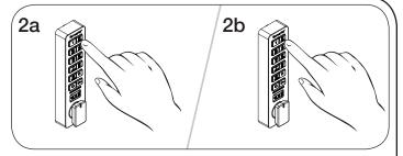
While the LED is on, press © [new 4-7 digit code] om.
