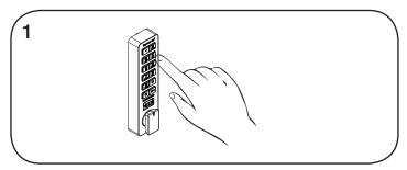
Go to a lock already programmed to operate with the Manager Keys. Press (2009) (811) (29),
