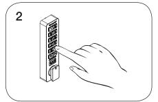
While the LED is on, press © [assigned user code] on
