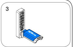
While the LED is on, insert a new User Key. Two sets of two-tone beeps will be heard and the LED will turn off.
