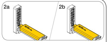
While the LED is flashing, insert the Programming Key.
