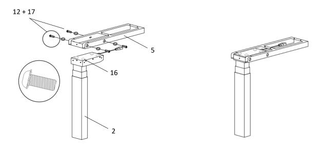
3. Install Side Support (Part 4) with Screw x2 (Part 12) and Star Washer x2 (Part 17) To Framework (Part 5).
